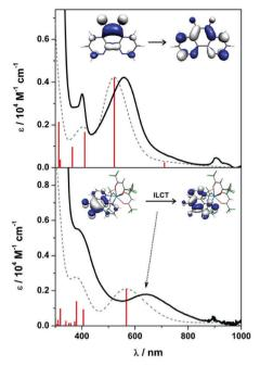
Fig. 4 Overlay of the experimental (solid line) and calculated (dashed line) electronic absorption spectra for  ${\bf 1}$  (top) and  ${\bf 3}$  (bottom) recorded at ambient temperature in MeCN. Vertical bars represent individual calculated transitions. Inset orbitals depict the donor/acceptor molecular orbitals (MO) that constitute the band at 558 nm in 1 and 639 nm in 3.
