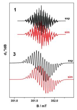
Fig. 2 Comparison of the X-band EPR spectrum of  $\bf 1$  (experimental conditions: frequency, 9.8461 GHz; power, 0.63 mW; modulation, 0.007 mT), and  $\bf 3$  at 293 K (experimental conditions: frequency, 9.8653 GHz; power, 0.63 mW; modulation, 0.02 mT) recorded in MeCN solution at 293 K. Experimental data are represented by the black lines and simulation depicted by the red traces.
