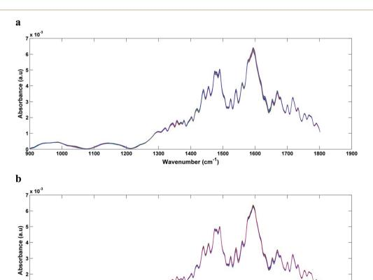
Wavenumber (cm<sup>-1</sup>) Fig. 2 Pre-processed spectra (cut between 900 and 1800 cm $^{-1}$ , baseline correction and smoothing) of: (a) DENV-3 in serum (1  $\times$  10 $^{3}$ , 1  $\times$  10 $^{2}$ , 1 and 0,1 PFU mL<sup>-1</sup>); (b) DENV-3 in blood (1  $\times$  10<sup>3</sup>, 1  $\times$  10<sup>2</sup>, 10 and 0,1 PFU mL<sup>-1</sup>).
