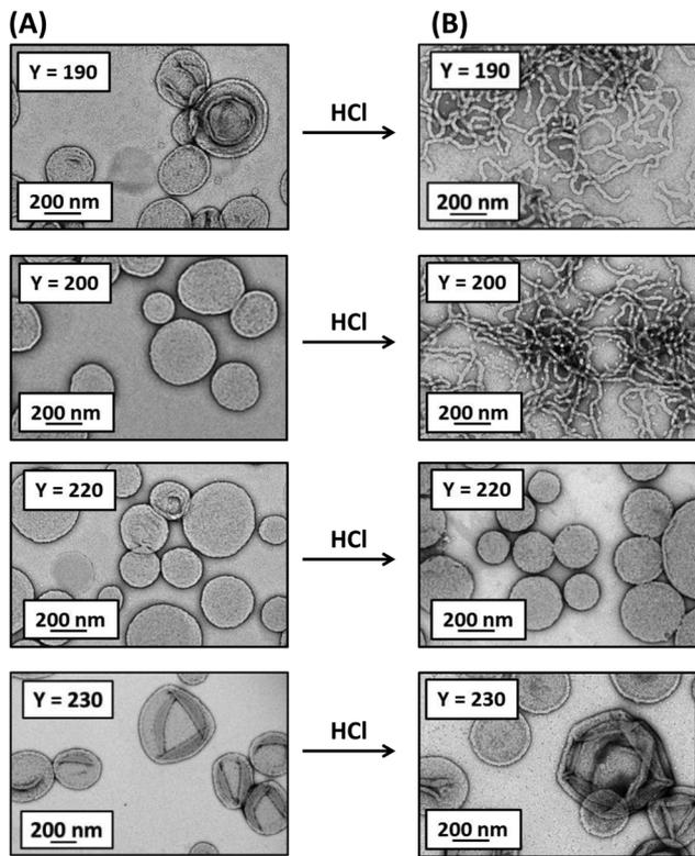
Fig. 2 Transmission electron microscopy images obtained for 0.1% w/w aqueous dispersions of MPETTC-PGMA<sub>43</sub>-PHPMA<sub>y</sub> ( $y = 190, 200, 220$  and  $230$ ) diblock copolymer nanoparticles at either (A) pH 7.0 or (B) pH 3.0. The pH switch was performed at 20 °C at 10% w/w copolymer concentration in each case.
