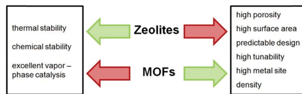
Fig. 6 Strengths (green) and weaknesses (red) of zeolites and MOFs, respectively. Modified from ref. 46.
