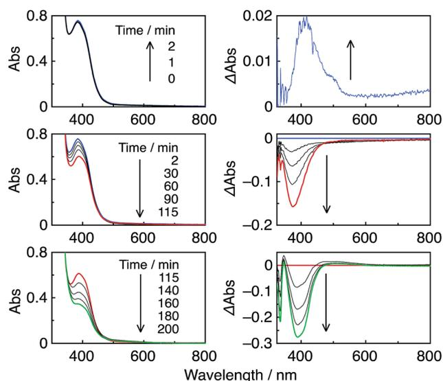
Fig. 5 UV-vis (left) and the corresponding differential absorption spectral changes (right) during the irradiation of a  $\text{CO}_2$ -saturated DMF-TEOA (5 : 1 v/v) solution containing **R(5)** (0.05 mM) as a PS and **Re-ACN** (0.05 mM) as the catalyst, under irradiation at  $\lambda_{\text{ex}} = 436 \text{ nm}$  ( $5.7 \times 10^{-9}$  einstein per s) in the initial stage (top) and over 3.5 h irradiation (middle and bottom).
