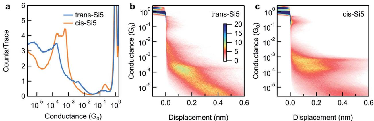
Fig. 3 (a) Logarithmically binned one-dimensional conductance histogram of *cis*-Si5 (orange) and *trans*-Si5 (blue). Histograms are made without data selection and normalized by the total number of traces. (b) and (c) Two-dimensional conductance histograms of *trans*-Si5 and *cis*-Si5 respectively, made from the same data as in (a).
