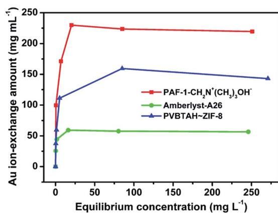
Fig. 3 Volumetric Au(i) adsorption isotherms for PAF-1-CH<sub>2</sub>-N<sup>+</sup>(CH<sub>3</sub>)<sub>3</sub>OH<sup>-</sup>, Amberlyst-A26 and PVBTAH-ZIF-8.
