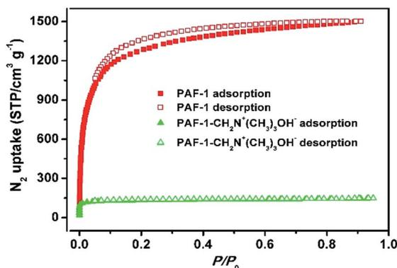
Fig. 1 N<sub>2</sub> sorption isotherms of PAF-1 (red) and PAF-1-CH<sub>2</sub>N<sup>+</sup>(CH<sub>3</sub>)<sub>3</sub>OH<sup>-</sup> (green).
