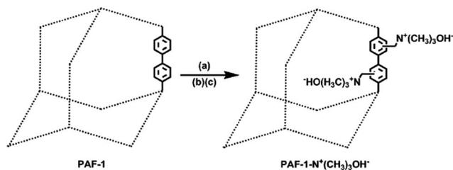
Scheme 2 Synthetic route of PAF-1-CH<sub>2</sub>N<sup>+</sup>(CH<sub>3</sub>)<sub>3</sub>OH<sup>-</sup>. (a) CH<sub>3</sub>-COOH/HCl/H<sub>3</sub>PO<sub>4</sub>/HCHO, 363 K, 3 days; (b) trimethylamine, ethanol, 353 K, 3 days; (c) 1 M NaOH, twice.
