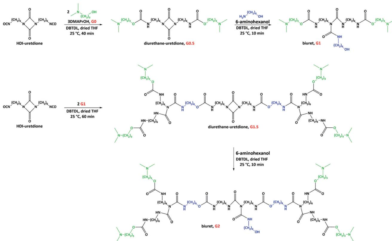
**Fig. 1** Reaction pathway for the preparation of the first and second generation of poly(urethane-biuret) dendrons with a hydroxyl focal point. HDI-uretdione: hexamethylene diisocyanate uretdione, 3DMAPrOH: 3-dimethylamino-1-propanol, DBTDL: dibutyltin dilaurate.
