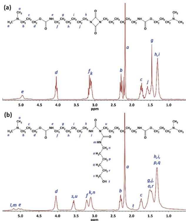
Fig. 2 <sup>1</sup>H-NMR spectra for G0.5 (a) and G1 (b) dendrons in CDCl<sub>3</sub>.
