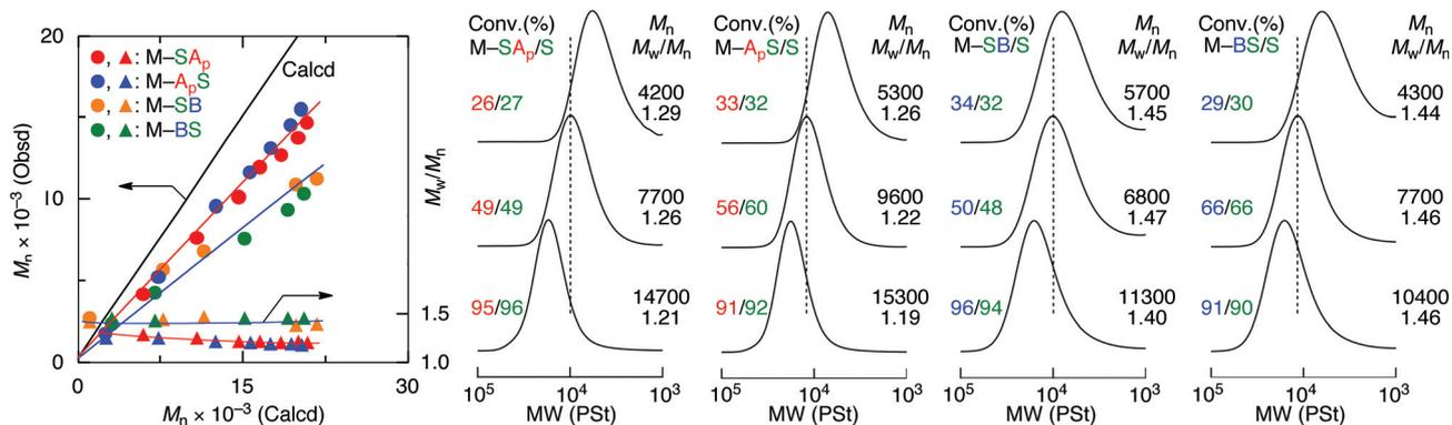
Fig. 4  $M_n$ ,  $M_w/M_n$ , and SEC curves for alternating RAFT copolymerization of a series of sequence-regulated functional oligomonomers and styrene in the presence of CDB as a RAFT agent.  $[M_1]_0 = [S]_0 = 1.0$  M,  $[CDB]_0 = 20$  mM.  $[AIBN]_0 = 20$  mM in toluene at 60 °C for M-SA<sub>p</sub> and M-A<sub>p</sub>S.  $[V-70]_0 = 20$  mM in PhC(CF<sub>3</sub>)<sub>2</sub>OH at 20 °C for M-SB and M-BS.
