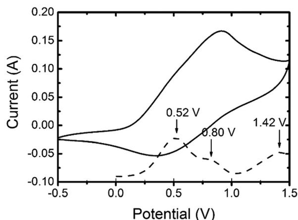
Fig. 3 Cyclic voltammetry (solid line) and differential pulse voltammetry (dotted line) of 3,6-Cbz-EDOT films on an ITO electrode, measured in  $\text{CH}_3\text{CN}$  with 0.1 M  $(n\text{C}_4\text{H}_9)_4\text{NPF}_6$  at the scan rate of 0.1 V s<sup>-1</sup> under flowing nitrogen.
