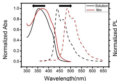
Fig. 2 Normalized UV-vis absorption and fluorescence spectra of 3,6-Cbz-EDOT in  $\text{CH}_2\text{Cl}_2$  measured at  $10^{-6}$  M repeat unit<sup>-1</sup> and in thin films.
