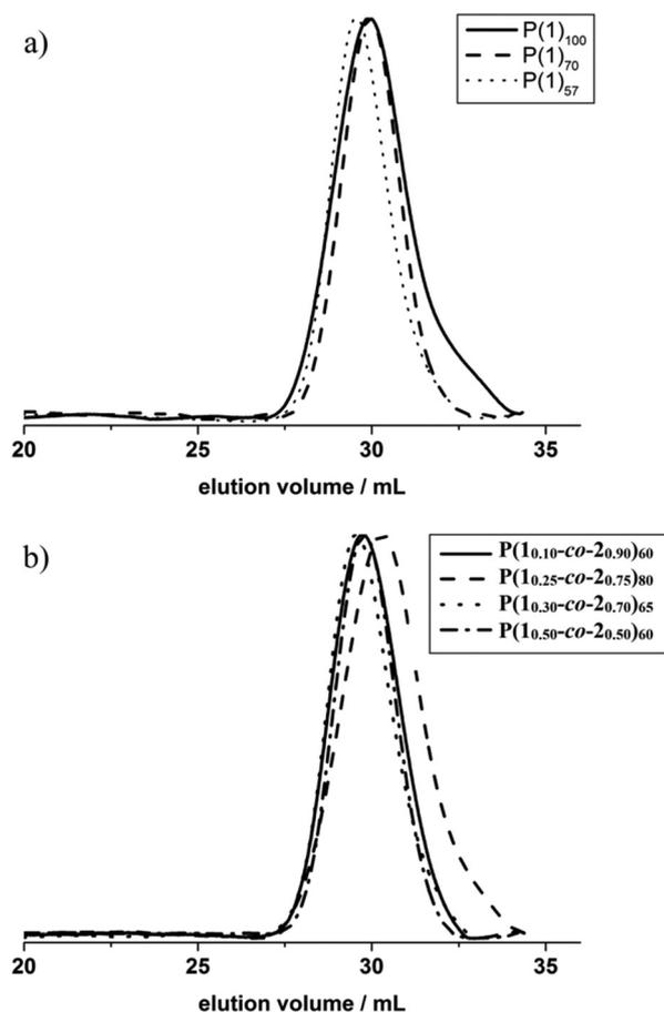
Fig. 2 SEC traces (RI detection) of (a)  $P(1)_n$  and (b)  $P(1_x\text{-co-}2_y)_n$  in DMF at 333 K (the indices  $x$  and  $y$  represent the relative copolymer composition whereas  $n$  represents the degree of polymerization).
