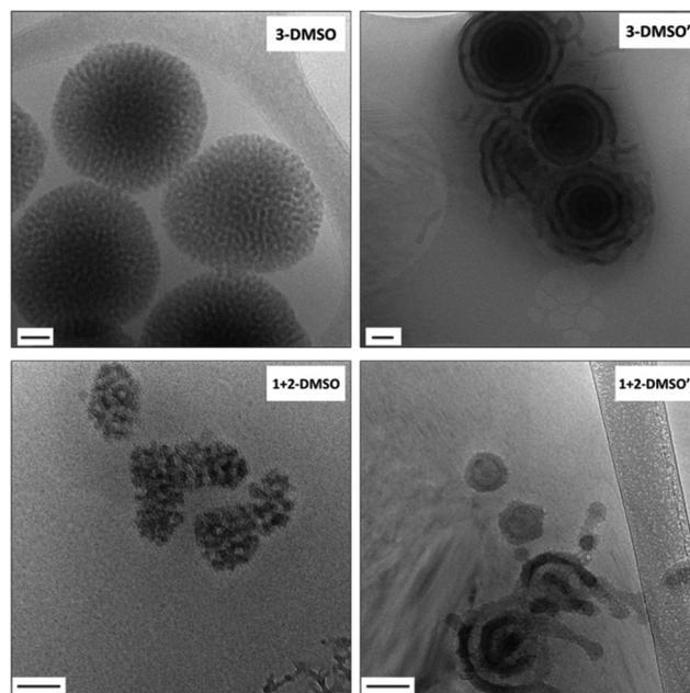
Fig. 2 Representative cryo-TEM images of self-assemblies 3-DMSO with a concentration of 1 mg mL<sup>-1</sup> and its annealed sample 3-DMSO' at 0.2 mg mL<sup>-1</sup>; 1 + 2-DMSO at a concentration of 1 mg mL<sup>-1</sup> and its annealed sample 1 + 2-DMSO' at 0.2 mg mL<sup>-1</sup>. Scale bar: 100 nm.
