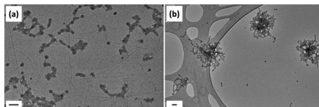
**Fig. 4** Representative unstained dry-state TEM images on GO grids of 3-DMSO annealed by different methods: (a) sample was heated at 60 °C for 45 min and then cooled down in an oil bath; (b) sample was heated from 15 °C to 60 °C and then cooled down from 60 °C to 15 °C at a rate of 1 °C min<sup>-1</sup> and repeated 3 times in total. Scale bar: 100 nm.
