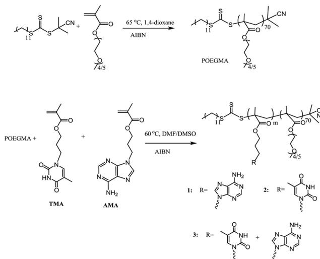
**Scheme 1** Synthetic route for the preparation of POEGMA<sub>70</sub> and the nucleobase-containing block copolymers, 1–3.
