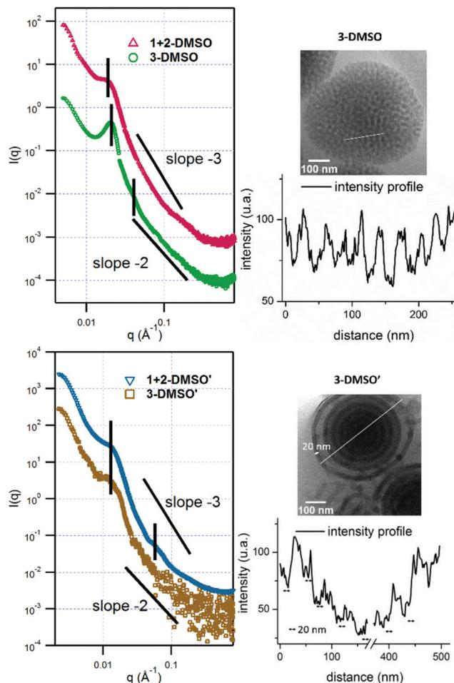
**Fig. 3** SAXS profiles of self-assemblies **3-DMSO**, **1 + 2-DMSO**, **3-DMSO'**, and **1 + 2-DMSO'**. The vertical black lines indicate the major peaks, indicative of the internal structure of the assemblies. The **1 + 2-DMSO** and **1 + 2-DMSO'** curves have been shifted by a factor 10 to improve clarity. Cryo-TEM images of **3-DMSO** and **3-DMSO'** and the corresponding intensity profile along the white line on the TEM images.
