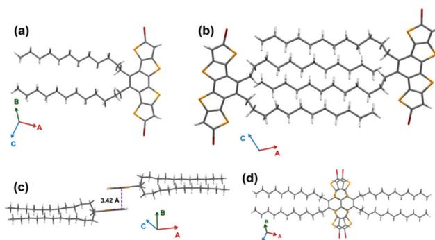
Fig. 2 Crystal structure and packing patterns of Br<sub>2</sub>-DTmBDT: (a) crystal structure, (b) alkyl chain interdigitation and close packing, (c)  $\pi$ - $\pi$  interactions in the dyad and (d) the top view of the dyad.
