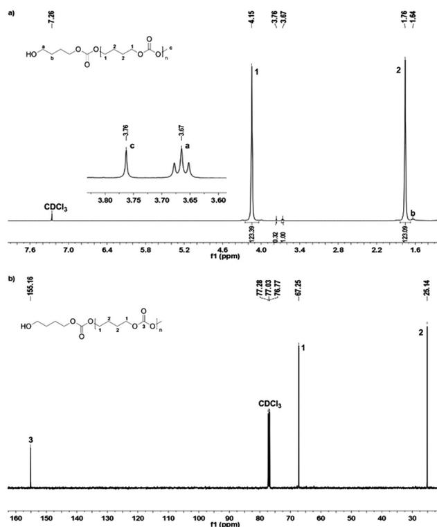
Fig. 2 <sup>1</sup>H (a) and <sup>13</sup>C NMR (b) spectra of PBC 9.
