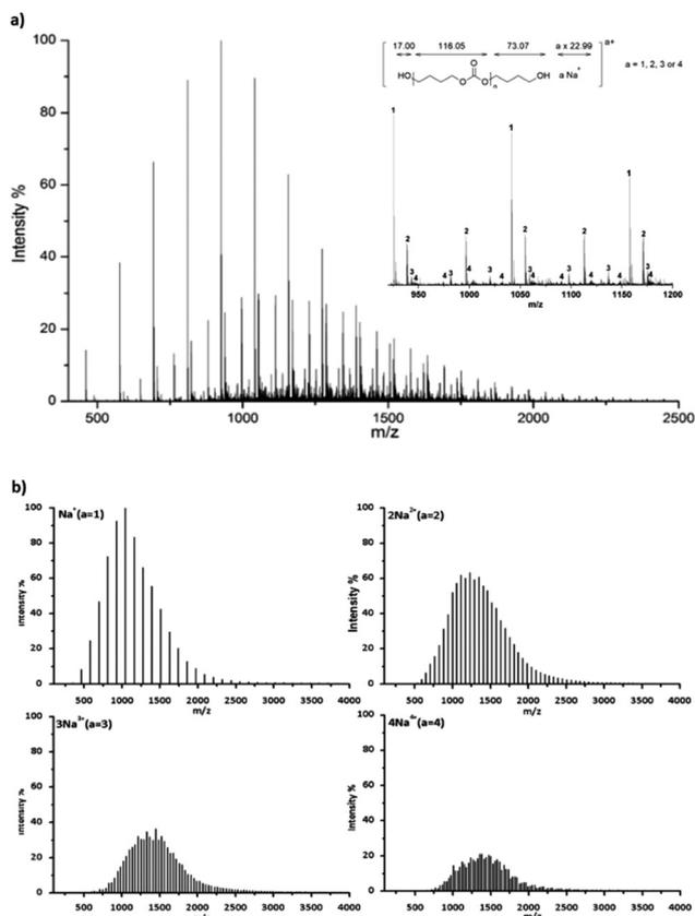
Fig. 4 ESI-TOF mass spectrum of PBC 7 (Table 2, entry 7) terminated with the hydroxyl group, (a) complete spectrum and a part of the spectrum distinguished by carrying charges  $a = 1, 2, 3$  and  $4$  in the region  $m/z$  400 to 2500, and (b) separated spectra with  $a = 1, 2, 3$  and  $4$ .
