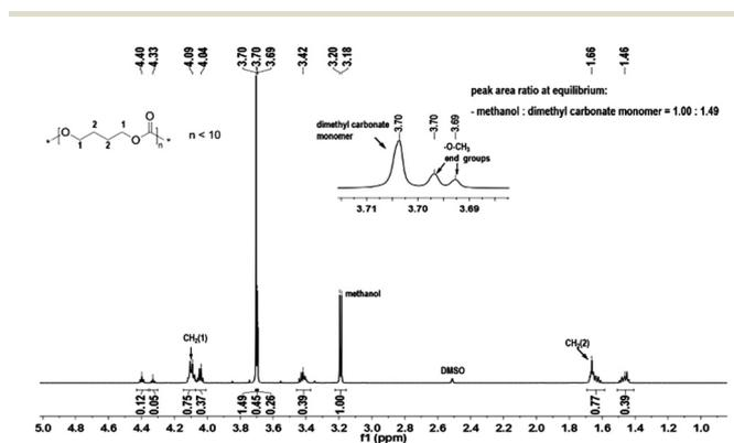
Fig. 1 <sup>1</sup>H NMR spectrum of the reaction solution of BD and DMC using cat. 1 at equilibrium.
