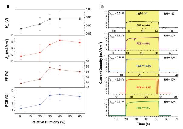
Fig. 6 (a) Average device performance characteristics (measured at a scan rate of 0.1 V s<sup>-1</sup>) as a function of relative humidity. Error bars represent plus or minus one standard deviation from the mean. (b) Steady-state current densities for representative devices at each relative humidity.
