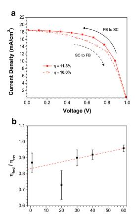
Fig. 5 (a) J-V curves measured at  $0.1\,\mathrm{V}\,\mathrm{s}^{-1}$  for the best device prepared at 40% RH. (b) Ratio of PCEs determined from forward (SC-FB) and reverse (SC-FB) scans as a function of RH. The linear fit is a guide to the eye.
