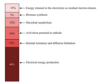
Fig. 7 Energy recovery in a glucose-fed microbial battery with an Ag<sub>2</sub>O/ Ag solid-state cathode (adapted with permission from ref. 120. Copyright 2013 PNAS).
