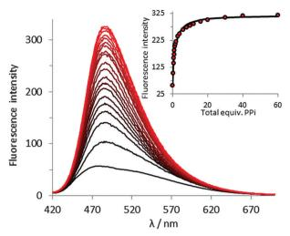
Fig. 4 Fluorescence emission spectra of  $1.2n_2$  (5  $\mu$ M) in response to PPI (0–300  $\mu$ M) in HEPES (5 mM, 145 mM NaCl, pH 7.4) at 25 °C.  $\lambda_{ex}$  = 390 nm, slits = 5 nm/5 nm. Inset: Binding isotherm (—) obtained by fitting the observed fluorescence intensities at 480 nm ( $\bullet$ ) to a 1:1 binding model using non-linear regression.
