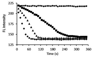
Fig. 5 Real-time assay of PPi (80  $\mu$ M) hydrolysis catalysed by different amounts of pyrophosphatase ( $\bullet$  = 0 units,  $\blacksquare$  = 0.5 units,  $\blacktriangle$  = 1.0 units,  $\bullet$  = 2.0 units) in the presence of  $\mathbf{3} \cdot \mathbf{Zn_2}$  (15  $\mu$ M) in Tris buffer (10 mM, 10 mM MqCl<sub>2</sub>, pH 7.5) at 30 °C,  $\lambda_{ex}$  = 390 nm, slits = 5 nm & 5 nm.
