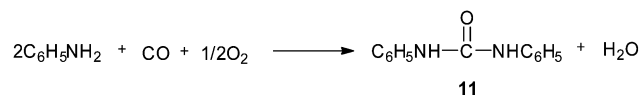
Scheme 5 Reagents and conditions: aniline (53.8 mmol), catalyst 5% Pd/C ( 5.0 \times 10^{-3} \text{ g cm}^{-3} ), NaI (0.87 mmol), DMF ( 95 \text{ cm}^3 ), CO : \text{O}_2 pressure (41 bar) (CO : \text{O}_2 , 5 : 1), temp. 100 °C, time 2 h.
