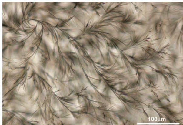
Fig. 36 POM image of the [BMIM][BF 4 ] gel combined with 1 wt% of DMBS. Reprinted with permission from ref. 216.
