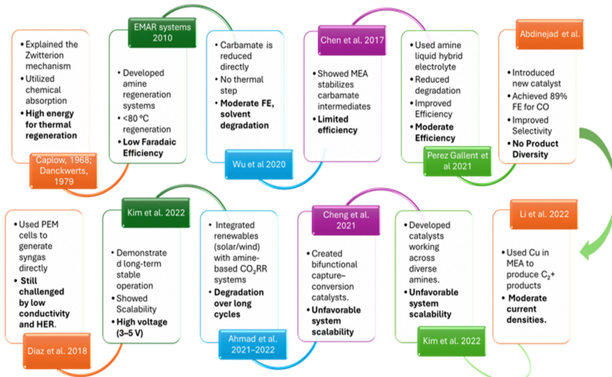
Fig. 56 A graphical timeline of the major developments in amine-based CO 2 capture and electrochemical conversion systems.
