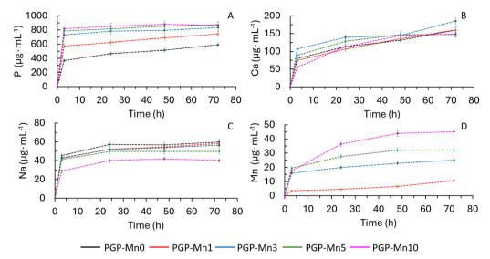
PGPs release of P (A), Ca (B), Na (C) and Mn (D) ions in DI water over 72 h
