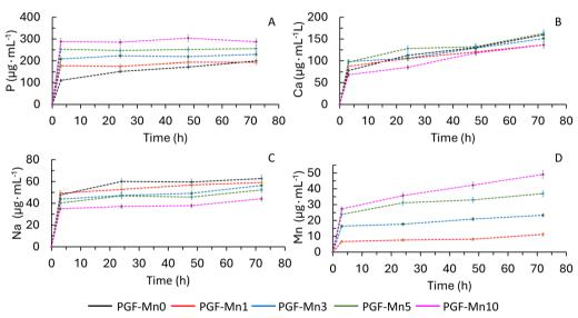
PGFs release of P (A), Ca (B), Na (C) and Mn (D) ions in DI water over 72 h
