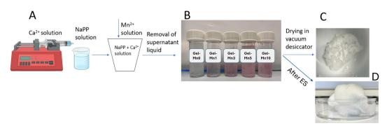
Fig. 1 (A) Schematic of the synthesis of PGs via coacervation; (B) images of all coacervate gels; (C) PGP-Mn0 in the system  $P_2O_5$ -CaO-Na<sub>2</sub>O obtained after drying of the coacervate Gel-Mn0 in a vacuum desiccator; (D) cotton-like bundle of PGF-Mn0 after ES of Gel-Mn0.
