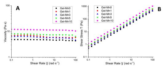
Fig. 2 Viscosity vs. shear rate (A) and shear stress vs. shear rate (B) of all polyphosphate coacervate gels
