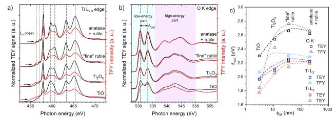
Fig. 7 Titanium L<sub>2.3</sub> (a) and oxygen K (b) edge X-ray absorption spectra after background subtraction, collected in TEY (black) and TFY (red) modes for TiO, Ti<sub>2</sub>O<sub>3</sub> and TiO<sub>2</sub> thin films with main line positions marked. Crystal field splitting  $\Delta_{oct}$  calculated as a difference in positions of eq and  $t_{2a}$  peaks based on O K and Ti  $L_{23}$  spectra in TEY and TFY modes (c) for thin films with different  $\phi_{M}$ .
