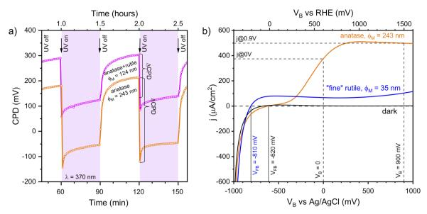
Fig. 8 Contact potential difference CPD vs. time for rutile/anatase and anatase thin films with changes under 370 nm illumination (\( \Delta CPD \)) marked (a); current density j as a function of applied bias voltage  $V_B$  in PEC (b).
