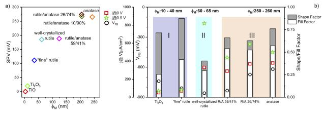
Fig. 9 Surface photovoltage SPV (= $-\Delta$ CPD) under 370 nm illumination as a function of figure of merit  $\phi_{\rm M}$  for thin films of different phase compositions (a) and the analysis of the most important parameters of PEC performance,  $V_{\rm FB}$  – flat band potential, j – current density upon white light illumination, shape and fill factor (b)
