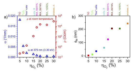
Fig. 3 Absorption coefficient (blue triangles) at  $\lambda = 375$  nm ( $h\nu = 3.30$  eV), electrical resistivity (red circles) from electrochemical impedance spectra measured at room temperature for titanium oxide thin films sputtered at different oxygen flow ratios  $\eta_{O_2}$  and oxygen partial pressures  $p_{O_2}$  (a), and figure of merit ( $\phi_M$ ) of thin films with different crystallographic structures calculated from eqn (3) (b).
