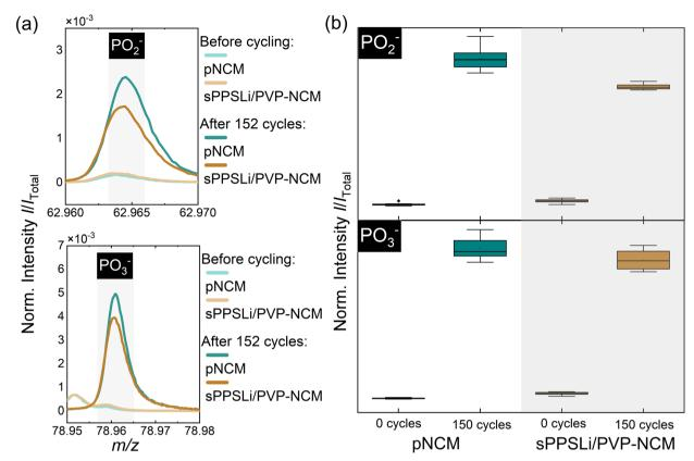
Fig. 6 (a) ToF-SIMS mass spectra for fragments that can be attributed to oxidative interfacial degradation products, such as  $PO_2^-$  and  $PO_3^-$  for pNCM and sPPSLi/PVP-NCM before cycling and after 152 cycles. (b) Corresponding boxplots of normalized intensities for degradation signals containing eight data points each.
