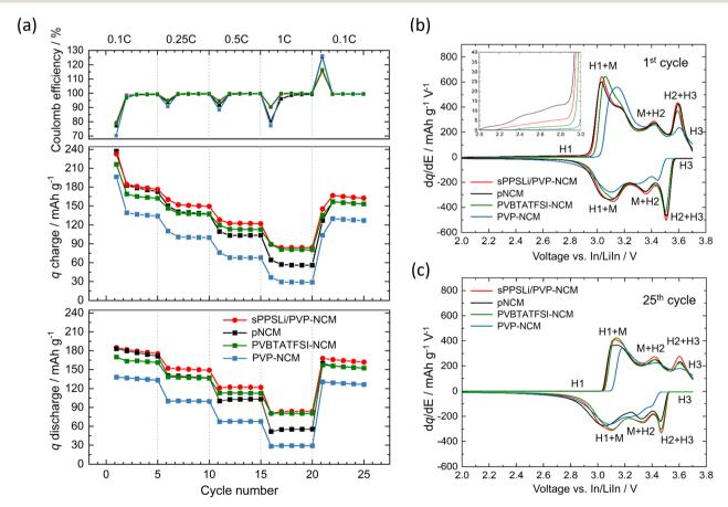
Fig. 3 (a) Specific capacity q and Coulomb efficiency at different C-rates of LilnSEBNCM using pNCM, sPPSLi/PVP-NCM, PVP-NCM, or PVBTATFSI-NCM, tested at C-rates of 0.1C to 1C in a pellet-type cell (Liln|Li<sub>6</sub>PS<sub>5</sub>Cl/VGCF/NCM) with 2.1 mA h cm<sup>-2</sup> nominal area capacity. Differential capacity dq/dE at 0.1C (b) in the 1st cycle and (c) in the 25th cycle. The inset in (b) shows an enlargement from 2–3 V (vs. In/Liln) of the 1st cycle.
