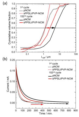
**Fig. 7** (a)  $L_{\rm diff}$  obtained using the EIS-PSD model for <sup>LiIn</sup>SEB<sup>pNCM</sup> and <sup>LiIn</sup>SEB<sup>sPPSLi/PVP-NCM</sup> in the 1st and 152nd cycles. The Warburg impedance is fitted through the EIS-PSD model to yield the cumulative volume fraction of particle size of different  $L_{diff}$ . (b) The chronoamperometry measurement shows the duration required for the current to drop below 2% of the initial charging current, which is proportional to  $L_{diff}$ .
