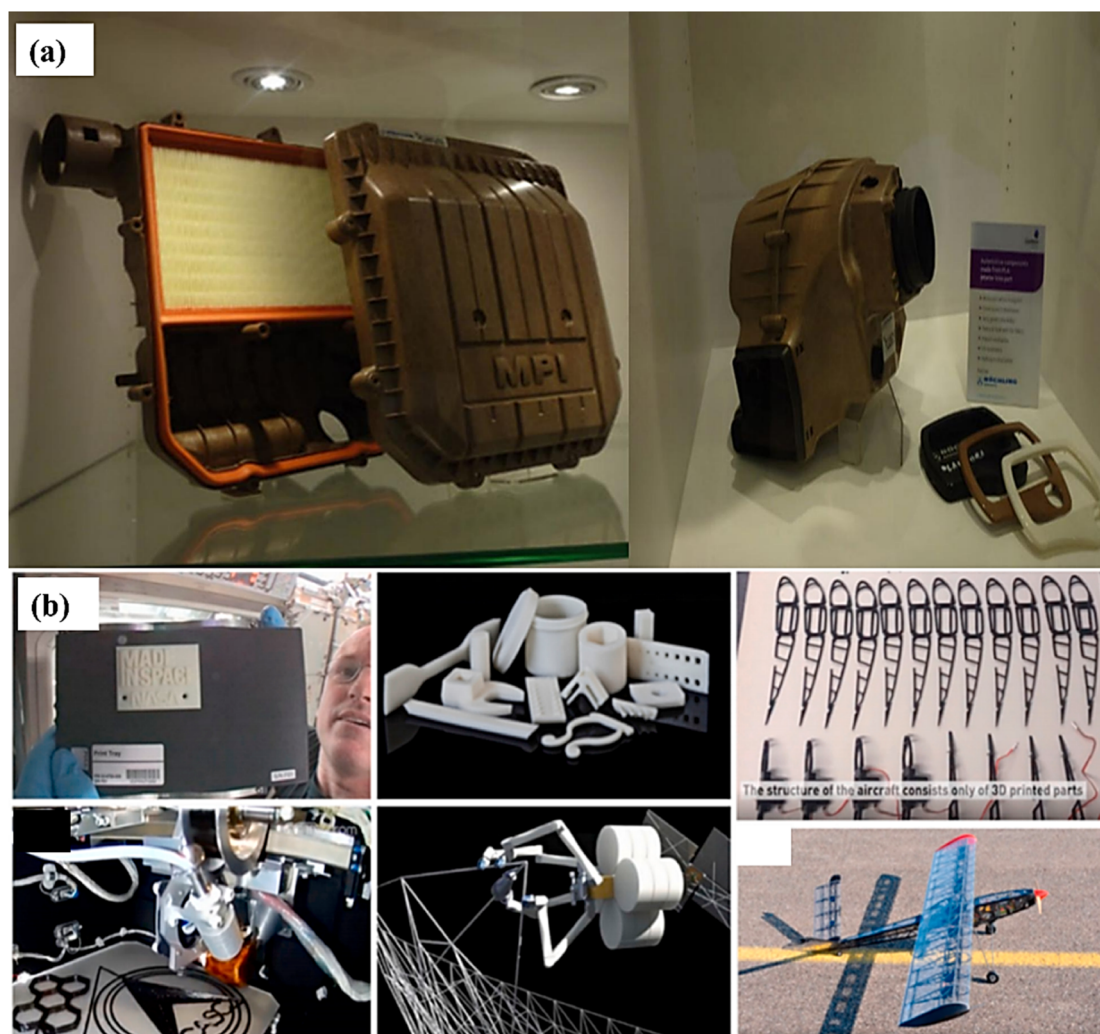
Fig. 8 (a) 3D printed air filter box and (b) space 3D printing and 3D printer parts from NASA's SpiderFab (reprinted with permission from ref. 18 and 123 Dananjaya S. A. V., Chevali V. S., Dear J. P., Potluri P., and Abeykoon C., 3D printing of biodegradable polymers and their composites-current state-of-the-art, properties, applications, and machine learning for potential future applications, Prog. Mater. Sci. , 2024, 101336 and Tuli N. T., Khatun S. and Rashid A. B., Unlocking the future of precision manufacturing: a comprehensive exploration of 3D printing with fiber-reinforced composites in aerospace, automotive, medical, and consumer industries, Heliyon , 2024, 10(5), e27328. Creative Commons Attribution 4.0 International License CC BY-NC-ND, https://creativecommons.org/licenses/by-nc-nd/4.0/ ).
