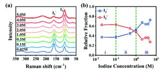
Fig. 11 (a) Raman spectra of PVA films dipped in KI/I<sub>2</sub> with different iodine concentrations. (b) Relative fraction of  $l_3^-$  and  $l_5^-$  obtained from peak deconvolution. Reprinted with permission from ref. 115; copyright 2021, the Royal Society of Chemistry.
