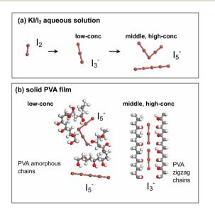
Fig. 10 Schematic of iodine species in (a) iodine solution, (b) solid PVA film, showing its distribution in the amorphous and crystalline regions of a PVA sample dipped in KI/I<sub>2</sub> solutions of different concentrations. Reprinted with permission from ref. 110; copyright 2015, the American Chemical Society
