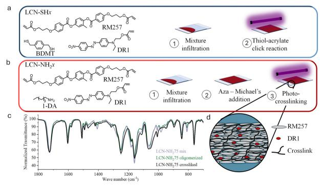
Fig. 1 Synthesis of LCNs. (a) Representation of the principal steps for the preparation of LCN-SHx and (b) LCN-NH2x. (c) ATR spectra of LCN-NH275 mixtures, LCN-NH<sub>2</sub>75 after Michael's oligomerization and LCN-NH<sub>2</sub>75 after photo-crosslinking reaction. (d) Representation of LCN structure at the molecular level.
