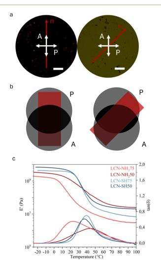
Fig. 2 Molecular alignment and mechanical tests on LCN films. (a) POM images of an LCN film with the director (n) oriented orthogonally to the polarisers and at  $45^{\circ}$ . Scale bar: 200  $\mu m$ . (b) Schematization of the transmittance of LCN films under two crossed polarizer (P) and analyser (A). (c) Storage modulus (E') and  $tan(\delta)$  representative curves for the LCNs
