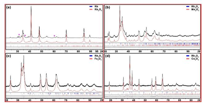
Fig. 3 Powder X-ray diffraction patterns of the residues obtained by thermal decomposition of [Rh(acac)<sub>3</sub>] (a) and molecular precursors 1–3 (b– d, respectively) with the Le-Bail fit. Black and red curves represent experimental and calculated patterns, respectively. Gray is the difference curve with theoretical peak positions shown as blue and red bars at the bottom. Impurity peaks are marked with asterisk
