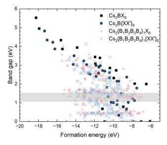
Fig. 2 DFT-calculated formation energy and band gap for 546 vacancy-ordered double perovskites including Cs<sub>2</sub>BX<sub>6</sub>, Cs<sub>2</sub>B{XX'}<sub>6</sub>,  $Cs_2\{B_1B_2B_3B_4\}_1X_6$ , and  $Cs_2\{B_1B_2B_3B_4\}_1\{XX'\}_6$ .
