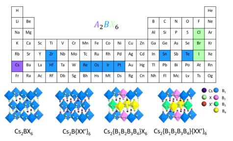
Fig. 1 The chemical space and atomic structures of the pure and mixed vacancy-ordered double perovskites investigated in this work.
