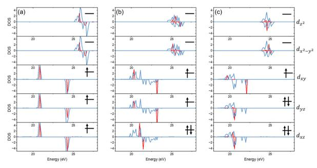
Fig. 4 (a) Comparison of the projected density of states on Re 5d orbitals in Cs<sub>2</sub>ReCl<sub>6</sub> (blue) and Cs<sub>2</sub>(ZrSnRePt)<sub>1</sub>Cl<sub>6</sub> (red). (b) Comparison of the projected density of states of Os 5d orbitals in Cs<sub>2</sub>OsCl<sub>6</sub> (blue) and Cs<sub>2</sub>(ZrSnOsPt)<sub>1</sub>Cl<sub>6</sub> (red). (c) Comparison of the projected density of states on Ir 5d orbitals in Cs2IrCl6 (blue) and Cs2{ZrSnIrPt}1Cl6 (red).
