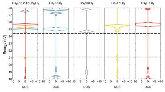
Fig. 5 Alignment of the density of states for the B-site-mixed Cs<sub>2</sub>(ZrSnTeHf)<sub>1</sub>Cl<sub>6</sub> perovskite and its constituent pure perovskites: Cs<sub>2</sub>ZrCl<sub>6</sub>, Cs<sub>2</sub>SnCl<sub>6</sub>, Cs<sub>2</sub>TeCl<sub>6</sub>, and Cs<sub>2</sub>HfCl<sub>6</sub>.
