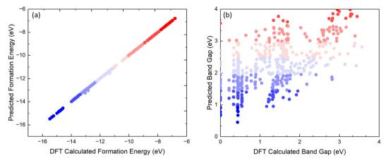
Fig. 3 The comparison between (a) the predicted formation energy from eqn (1) and the DFT-calculated formation energy and (b) the predicted band gap from eqn (2) and the DFT-calculated band gap.
