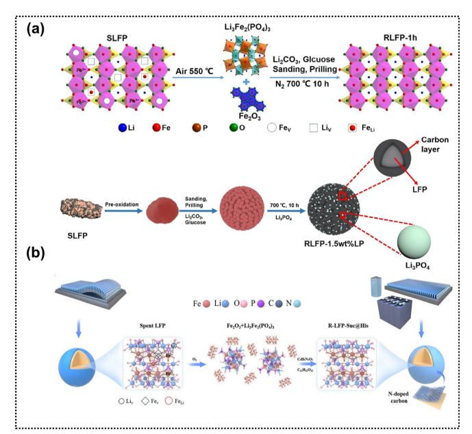
Fig. 5 (a) Schematic of cooperative RLFP. Reproduced from ref. 62, Copyright 2024, with permission from the American Chemical Society. (b) Schematic of the regeneration of SLFP batteries. Reproduced from ref. 63, Copyright 2024, with permission from the Royal Society of Chemistry.
