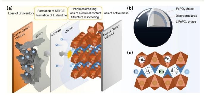
Fig. 2 (a-c) Degradation mechanism of LFP cathode materials. Reproduced from ref. 17, Copyright 2024, with permission from Elsevier.
