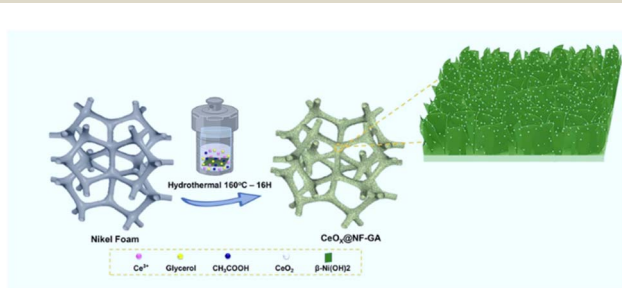
Scheme 1 Schematic of the synthesis of the Ce@NF-GA sample.
