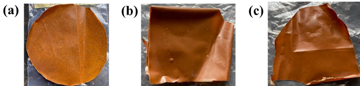
Fig. 9 Synthesized (a) MPVA/1BXT:1AC, (b) MPVA/1BXT:2AC and (c) MPVA/2BXT:1AC membranes.
