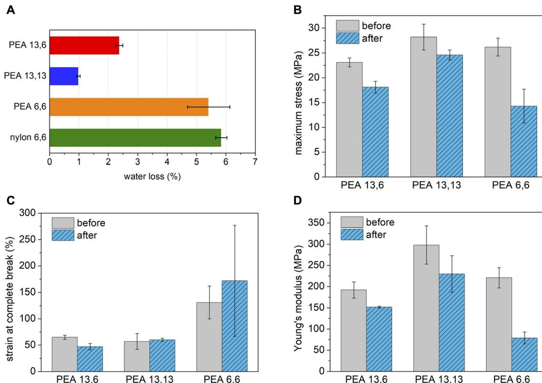
**Fig. 2** (A) Amount of DI water absorbed in 24 hours by PEAs and nylon 6,6, as determined by mass loss at 100 °C over 2 hours (TGA). The maximum stress (B), percent strain at break (C), and Young's modulus (D) of PEAs before and after storing samples in DI water for 24 hours.
