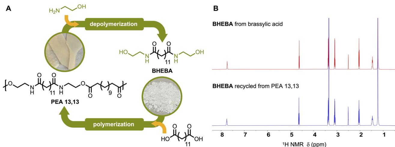
**Fig. 5** (A) Chemical recycling of PEA 13,13 *via* aminolytic depolymerization and esterification polymerization. (B) <sup>1</sup>H NMR (in DMSO- $d_6$ ) comparison of BHEBA synthesized from brassylic acid (top) and BHEBA obtained *via* aminolytic depolymerization of PEA 13,13 (bottom).
