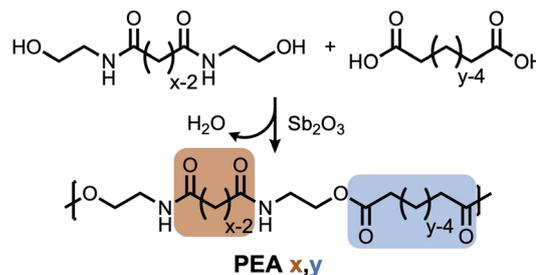
**Scheme 2** General representation of PEAs (polyesteramides) synthesized in this study. The number of carbons between amide N atoms is given by  $x$ . The number of carbons between ester O atoms is given by  $y$ .
