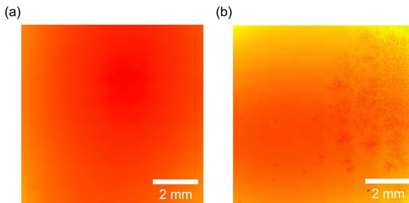
**Fig. 6** White light interference micrographs of the perovskite layer spin-coated under the optimized conditions (a) and reference conditions (b).
