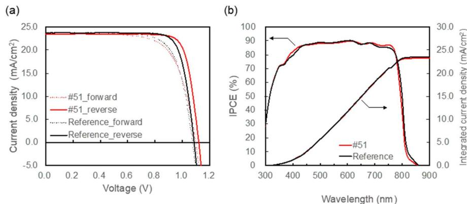
Fig. 7 (a)  $J$ - $V$  curves for devices fabricated under the optimized condition (#51) (red line) and reference condition (black line). (b) IPCE spectra for devices fabricated under the optimized condition (#51) (red line) and reference condition (black line).
