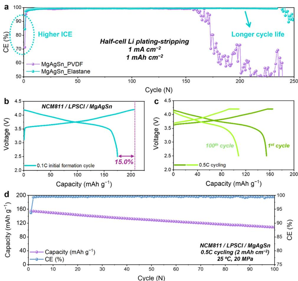
**Fig. 6** Half-cell and full-cell performances of the MgAgSn anode-less electrodes. (a) CE comparison during Li plating–stripping tests in half-cells. (b–d) Full-cell performance of the MgAgSn anode-less electrodes with the Elastane binder, paired with an NCM811 cathode: (b) voltage profile during the initial 0.1C formation cycle; (c) voltage profiles and (d) cycling performance at 0.5C (1C = 2 mA cm<sup>-2</sup>).
