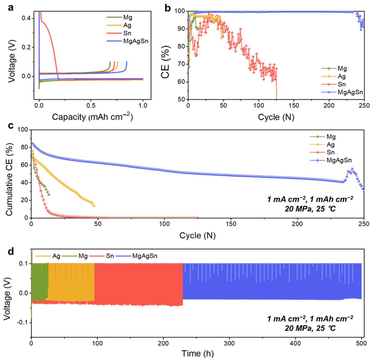
**Fig. 2** Half-cell Li plating–stripping evaluations of the single- and multi-seed anode-less electrodes. (a) Voltage profiles of the first cycle. (b) Coulombic efficiencies (CEs), (c) cumulative CE, and (d) voltage–time profiles of the half-cells over cycling.
