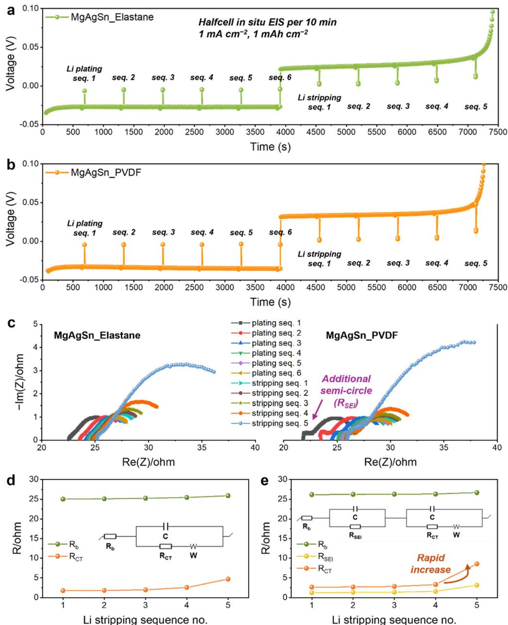
**Fig. 5** *In situ* EIS analysis during Li plating–stripping in the half-cell. (a and b) Voltage profiles during the EIS measurements of the MgAgSn half-cells with the (a) Elastane and (b) PVDF binders. (c) Nyquist plots representing the EIS results. (d and e) Resistance values and corresponding equivalent circuit models used for EIS data fitting of the MgAgSn half-cells with the (d) Elastane and (e) PVDF binders.
