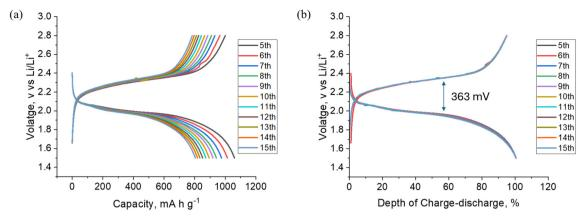
Fig. 8 Overvoltage analysis of Li-S cell: (a) voltage versus real charge-discharge capacity and (b) voltage versus depth of charge-discharge capacity profiles of the Li-S cell having 30 mol% LiTFSI in P<sub>111i4</sub>FSI IL-electrolyte.
