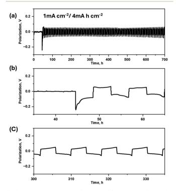
Fig. 1 Li metal symmetric cell cycling: (a) voltage profiles during lithium plating/stripping processes in Li|Li symmetrical cells containing 30 mol% LiTFSI in P<sub>111i4</sub>FSI electrolytes at current density 1.0 mA cm<sup>-2</sup> (4 mA h cm<sup>-2</sup>), at 50 °C (b) and (c) are the zoomed view.
