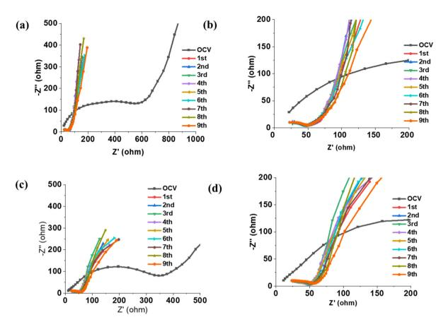
Fig. 6 Electrochemical impedance spectroscopy of LiS cell (15 wt% CMC, 21 wt% HSAC, 14 wt% C65 and 50 wt% S) at OCV and after lithiation in (a) 30 mol% LiTFSI in P<sub>111i4</sub>FSI IL and (c) 50 mol% LiFSI in P<sub>111i4</sub>FSI FSI IL electrolyte. (b, and d) are the zoomed view of (a, and c) respectively.
