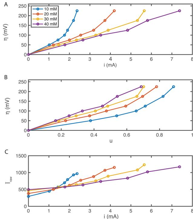
Fig. 4 Characteristic plots from MSC experiments. (A) Polarization plot as a result of the MSC experiment for  $[\text{AQDS}]_0$  values indicated. (B) Applied overpotentials as function of the electrolyte utilization  $u$ . (C) Mean raw fluorescence intensity  $\bar{I}_{\text{raw}}$  averaged over the entire confocal microscope image as a function of the current  $i$ .
