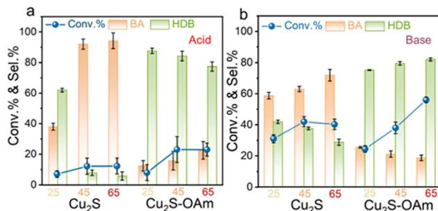
Fig. 5 BZH conversion and selectivity toward BA and HDB after 20 min reaction on  $\text{Cu}_2\text{S}$  and  $\text{Cu}_2\text{S}$ -OAm electrodes at  $-0.8$  V vs. RHE,  $25$  °C,  $45$  °C or  $65$  °C in (a) 1 M sodium acetate-acetic acid solution (pH = 5.2) with 20 mM BZH; (b) 1 M potassium carbonate-potassium bicarbonate solution (pH = 9.0) with 20 mM BZH.
