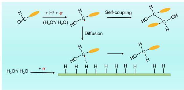
**Scheme 1** Two pathways for the BZH electroreduction, to BA or HDB. The orange ellipsoid represents the benzene ring. Red spots represent electrons provided by the electrode that is represented here by a green bar.
