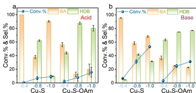
Fig. 4 BZH conversion and selectivity toward BA and HDB after 20 min reaction on  $\text{Cu}_2\text{S}$  and  $\text{Cu}_2\text{S}$ -OAm electrodes at 0.4,  $-0.8$ ,  $-1.0$  V vs. RHE,  $25$  °C in (a) 1 M sodium acetate-acetic acid solution (pH = 5.2) with 20 mM BZH; (b) 1 M potassium carbonate-potassium bicarbonate solution (pH = 9.0) with 20 mM BZH.
