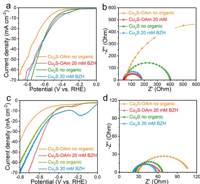
**Fig. 3** (a) LSV curves and (b) Nyquist plots at  $-0.7$  V vs. RHE of  $\text{Cu}_2\text{S-OAm}$  and  $\text{Cu}_2\text{S}$  in 1 M sodium acetate-acetic acid electrolyte ( $\text{pH} = 5.2$ ) with and without BZH at room temperature; (c) LSV curves and (d) Nyquist plot at  $-0.7$  V vs. RHE of  $\text{Cu}_2\text{S-OAm}$  and  $\text{Cu}_2\text{S}$  in 1 M potassium carbonate-potassium bicarbonate electrolyte ( $\text{pH} = 9$ ) with or without BZH at room temperature.
