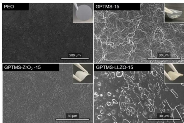
Fig. 9 SEM images and digital photos (top right) of PEO SPE with smooth surface, GPTMS 15% CPE with fibrous and uneven structure, GPTMS–ZrO<sub>2</sub> 15% CPE with homogeneous surface and a uniform distribution of particles, and GPTMS–LLZO 15% CPE with heterogeneous surface and large particle agglomerates.
