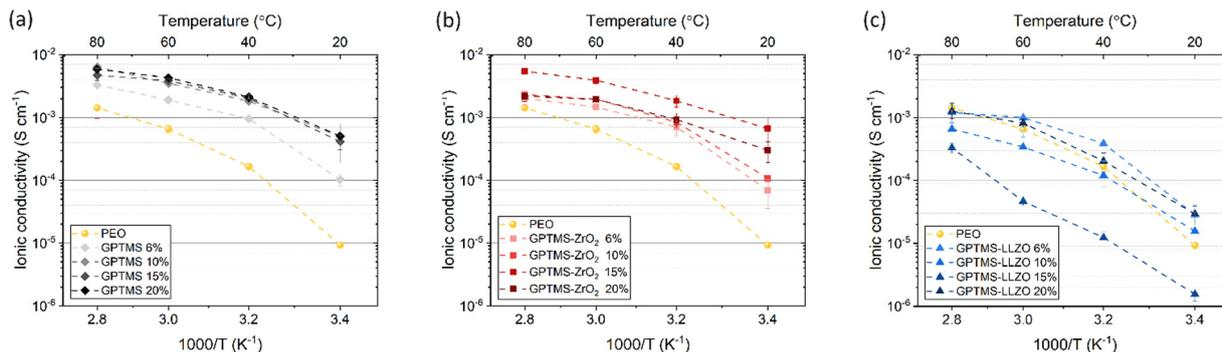
Fig. 6 Ionic conductivity of 6, 10, 15, 20 vol% of (a) GPTMS CPE, (b) GPTMS–ZrO<sub>2</sub> CPE and (c) GPTMS–LLZO CPE measured at 20, 40, 60, and 80 °C in comparison of PEO SE.
