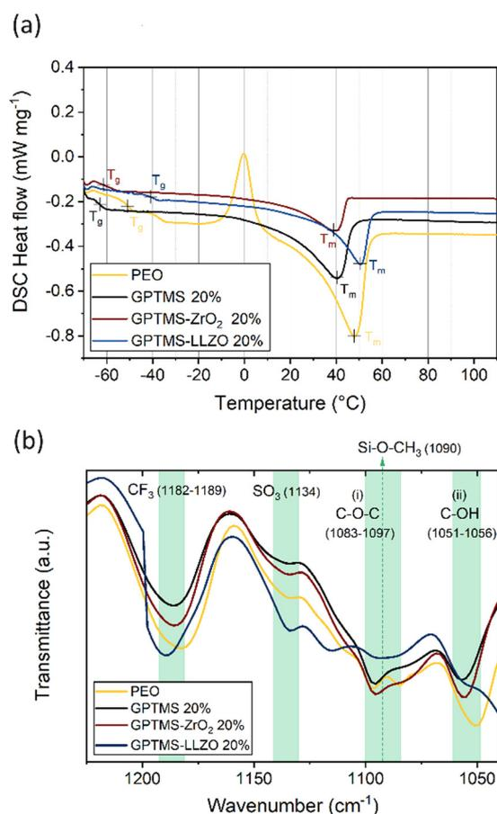
Fig. 4 (a) The second heating curves of the DSC measurements and (b) FT-IR spectra of the PEO-LiTFSI SE, filler-free GPTMS 20% CPE, GPTMS-ZrO<sub>2</sub> 20% CPE, and GPTMS-LLZO 20% CPE.
