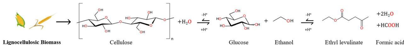
Fig. 1 Reaction mechanism for the production of ethyl levulinate from lignocellulosic biomass.<sup>14</sup> The primary objective of these conversion processes is the elimination of the covalently bounded oxygen atoms (in red) to produce a liquid enriched in hydrogen and carbon, such as ethyl levulinate.
