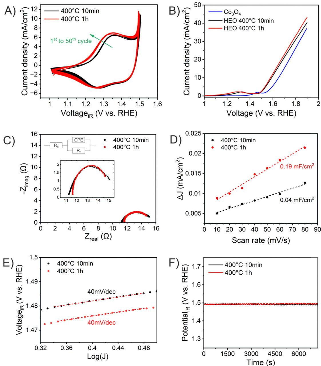
**Fig. 3** Electrochemical performance of HEO-400-10min (black) and HEO-400-1h (red): (A) cyclic voltammograms, (B) linear sweep voltammetry, (C) Nyquist plots measured at 1.6 V vs. RHE, (D) differential current densities and the corresponding the double-layer capacities,  $C_{DL}$ , determined by linear fitting, (E) Tafel plots, and (F) chronopotentiometry analysis performed at  $10 \text{ mA cm}^{-2}$  for 2 hours. All experiments were conducted in 1 M KOH (pH  $\approx$  13.6).
