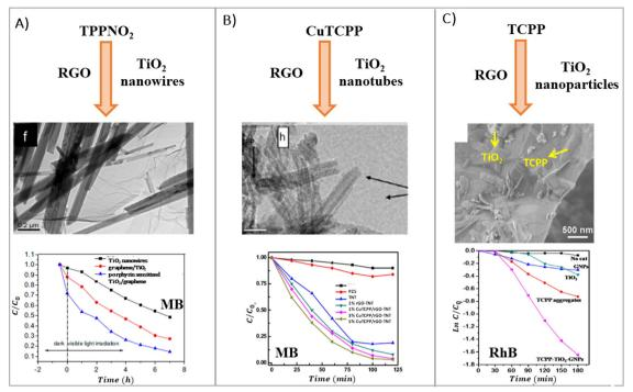
Fig. 30 Ternary nanostructures of various porphyrin/RGO/TiO<sub>2</sub> composites and their photocatalytic performance. Adapted with permission from ref. 149, 151 and 153. Copyright 2014 Elsevier B.V, 2016 Hydrogen Energy Publications LLC, 2015 Elsevier Inc.
