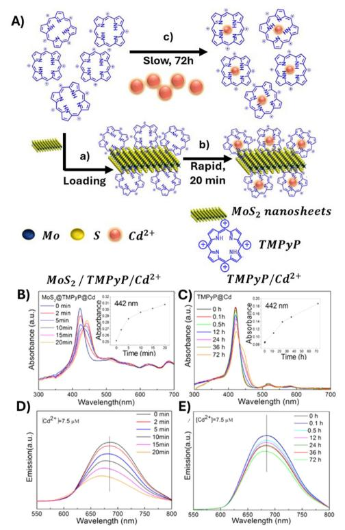
Fig. 43 (A) Schematic showing the strategy for removing  $Cd^{2+}$  using TMPyP self-assembled with  $MoS_2$  nanosheets. (B) Time-dependent UV-vis absorption spectra of MoS<sub>2</sub>/TMPyP/Cd<sup>2+</sup> and (C) TMPyP with Cd<sup>2+</sup>; insets: plots of the absorbance at 442 nm versus reaction time. (D) Time-dependent emission spectra of MoS<sub>2</sub>/TMPyP/Cd<sup>2+</sup> and (E) TMPyP/Cd<sup>2+</sup>. Reproduced from ref. 55. Copyright 2017 American Chemical Society.
