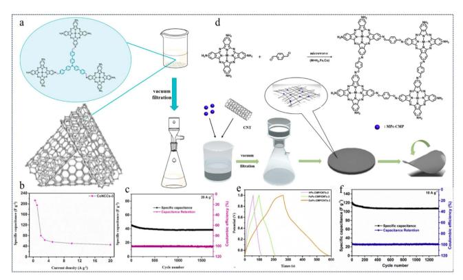
Fig. 22 (a) Schematic preparation process for MNCCs (M=Co, Fe). (b) Specific capacitances of CoNCCs-3 at different current densities. (c) Cycling performance and coulombic efficiency of CoNCCs-3 at 20 A  $g^{-1.136}$  Copyright 2021, Elsevier. (d) Synthetic process of MPc-CMP/CNTs. (e) GCD curves of MPc-CMP/CNTs-2 (M =  $H_2$ , Co, Fe) obtained at 1 A  $g^{-1}$ . (f) Cycling performance and coulombic efficiency of CoPc-CMP/ CNTs-2 at 10 A g<sup>-1</sup>.142 Copyright 2020, Elsevier.
