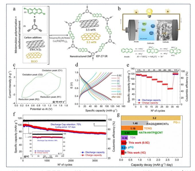
Fig. 15 (a) Synthesis strategy for IEP-27-SR mixtures. (b) Scheme of the aluminium-phenazine battery. (c) CV recorded at 10 mV s $^{-1}$ . (d) GCD profiles of the Al//IEP-27-SR battery. (e) Battery rate performance. (f) Long-term cycle stability of an Al//IEP-27-SR battery. (g) Capacity fade per day.107 Copyright 2023, Royal Society of Chemistry.
