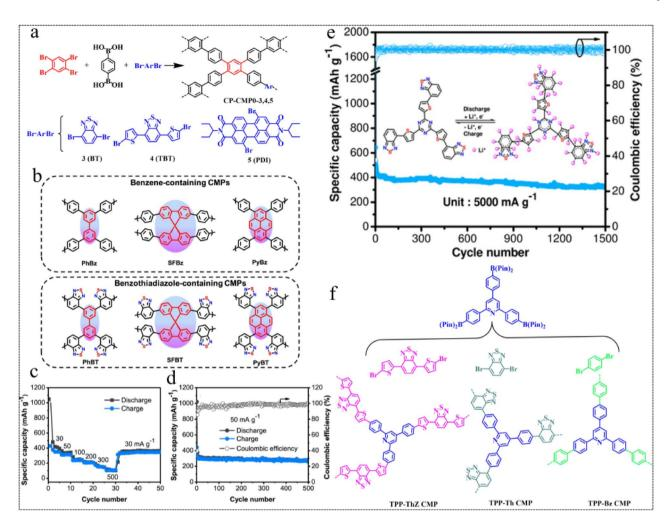
Fig. 3 Suzuki-Miyaura coupling reaction routes. (a) Synthesis of CP-CMP0, 3, 4, 5.48 Copyright 2016, American Chemical Society. (b) Polymer structures. (c) Rate performance of PyBT. (d) Cycling stability and coulombic efficiency of PyBT. 49 Copyright 2019, American Chemical Society. (e) Electrochemical performance graph of the TzThBT polymer.50 Copyright 2020, Wiley. (f) Synthesis and chemical structures of the TPP-based CMPs.51 Copyright 2023, Royal Society of Chemistry.
