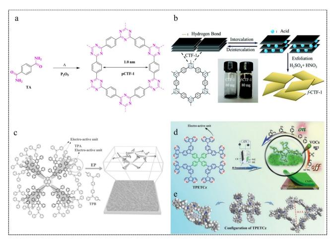
Fig. 8 (a) Synthesis of pCTF-1.75 Copyright 2018, Wiley. (b) Preparation process of f-CTF-1 nanosheets.76 Copyright 2019, Royal Society of Chemistry. (c) Dimerisation of TPA with TPB and schematic representation of the crosslinked network microstructure of EP membranes.80 Copyright 2016, Wiley. (d) EP preparation of TPETCz-CMP films. (e) Structural model of TPETCz-CMP.26 Copyright 2020, Wiley.
