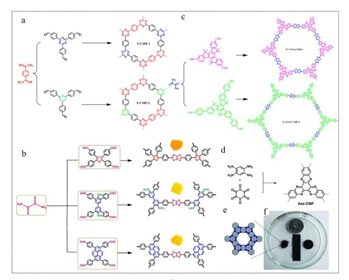
Fig. 7 Heterocycle linkages. (a) Synthesis of T-CMP-1 and TCMP-2.<sup>69</sup> Copyright 2021 American Chemical Society. (b) Synthesis of Ts-ThTh-CMP, Bi-ThTh-CMP, and Py-ThTh-CMP.70 Copyright 2022, Elsevier. (c) Synthesis of Tx-TzTz-CMP-1 and TxTzTz-CMP-2.71 Copyright 2023, American Chemical Society. (d) Synthesis of Aza-CMP. (e) The elementary pore structure of Aza-CMP. (f) Photographic image of different shapes of Aza-CMPs.<sup>72</sup> Copyright 2019, Royal Society of Chemistry.
