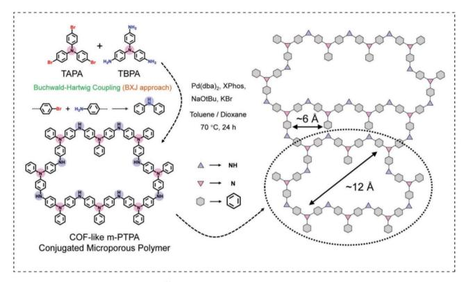
Fig. 14 The synthesis route of COF-like m-PTPA.<sup>106</sup> Copyright 2021, Wiley.
