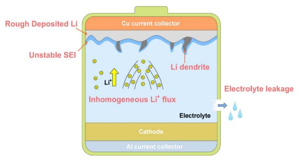
Fig. 15 Challenges of anode-free lithium metal batteries.
