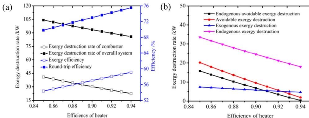
Fig. 12 (a) The effect of turbine efficiency on SC-CCES under traditional turbine analysis; (b) the effect of turbine efficiency on SC-CCES under advanced turbine analysis.<sup>80</sup>
