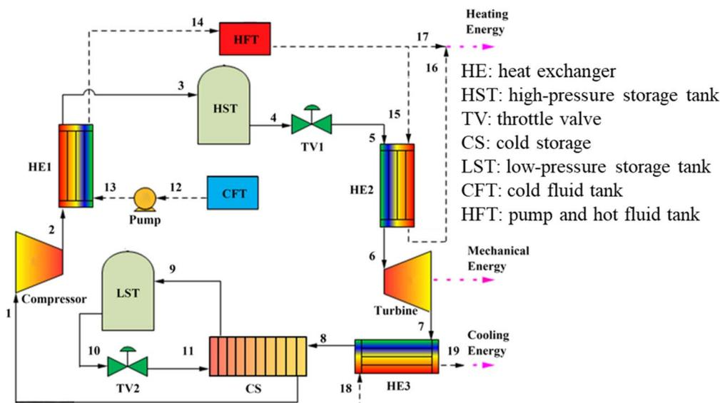
Fig. 3 Schematic diagram of CCES system.<sup>46</sup>
