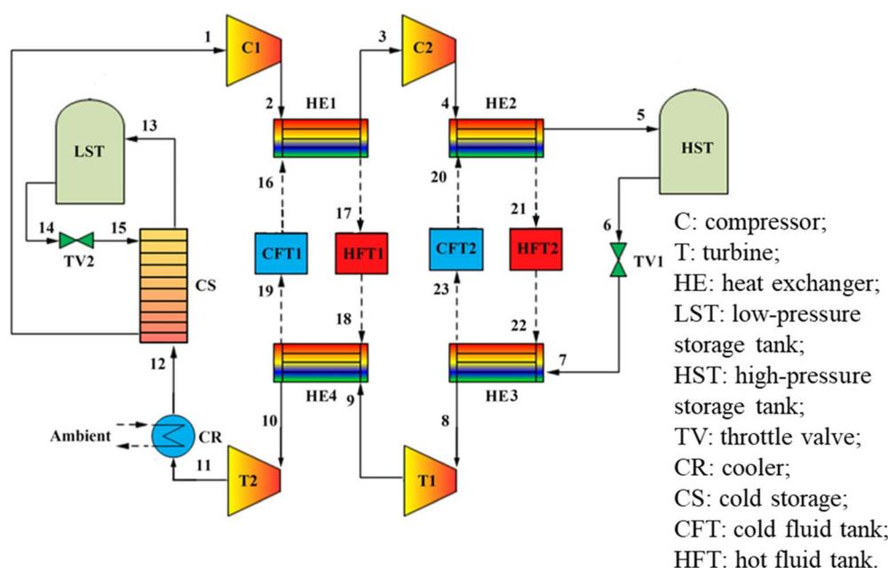
Fig. 6 A new triple production system based on transcritical Brayton cycle and carbon dioxide energy storage.<sup>62</sup>
