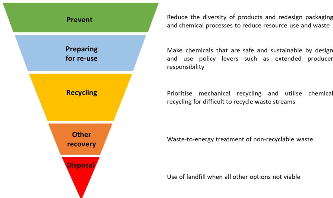
Fig. 2 Applying the waste hierarchy principle to the chemical sector, reproduced from ref. 14 with permission from <https://www.gov.uk/>, copyright 2011.<sup>14</sup>
