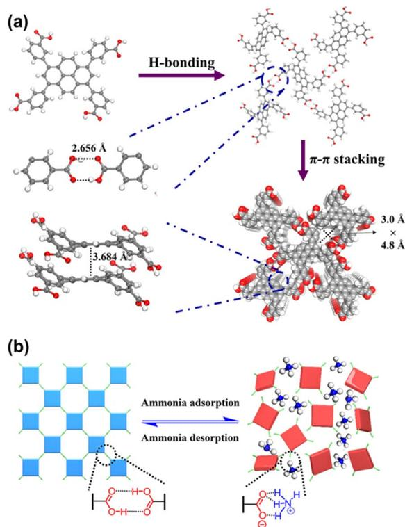
Fig. 8 (a) Crystal structures of FDU-HOF-3; (b) schematic illustration of the self-healing effect of FDU-HOF-3 before and after  $\text{NH}_3$  capture.<sup>64</sup>
