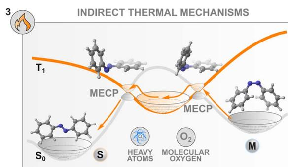
Fig. 6 The mechanism of thermal isomerisation of azobenzene involves crossing to the  $T_1$  state via two minimum energy crossing points (MECPs). The presence of heavy atoms and molecular oxygen influence the thermal process.
