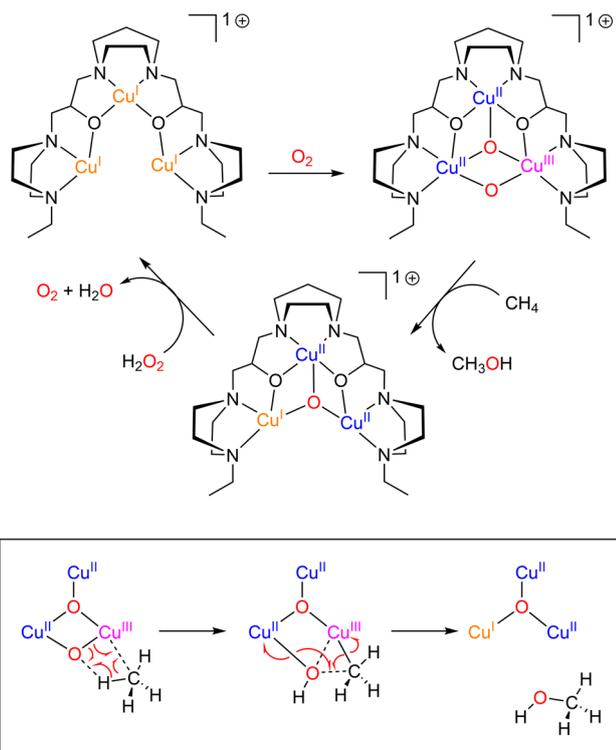
Scheme 13 Top: Catalytic cycle for the oxidation of CH<sub>4</sub> mediated by the  $[\text{Cu}^{\text{I}}\text{Cu}^{\text{I}}\text{Cu}^{\text{I}}(7\text{-}N\text{-Etpyz})]^{1+}$  complex and O<sub>2</sub> in the presence of hydrogen peroxide. Bottom: Proposed intermediates for methane oxidation. Adapted from ref. 227 and 229.
