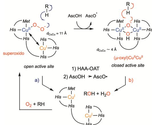
**Scheme 2** Recently revisited mechanism for PHM and DβH showing the mechanisms involving an HAA by (a) Cu<sub>M</sub>-superoxido intermediate in an open dicopper active site and (b) μ-oxyl dicopper intermediate in closed dicopper active site. Abbreviation: AscOH for ascorbic acid.
