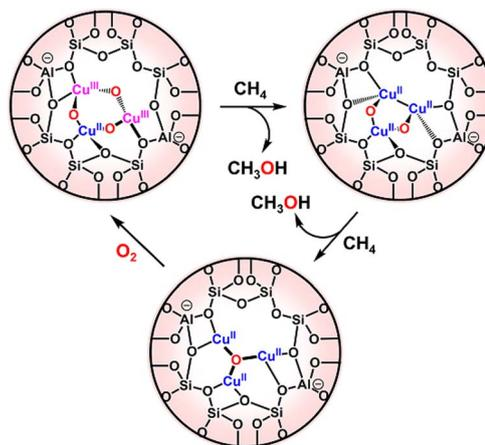
Fig. 16 Formation of a [Cu<sub>3</sub>(μ<sub>3</sub>-O)]<sup>2+</sup> species and two CH<sub>3</sub>OH molecules from the reaction of CH<sub>4</sub> with [Cu<sub>2</sub>(μ-O)]<sup>2+</sup> in MOR zeolite. Adapted from ref. 252.
