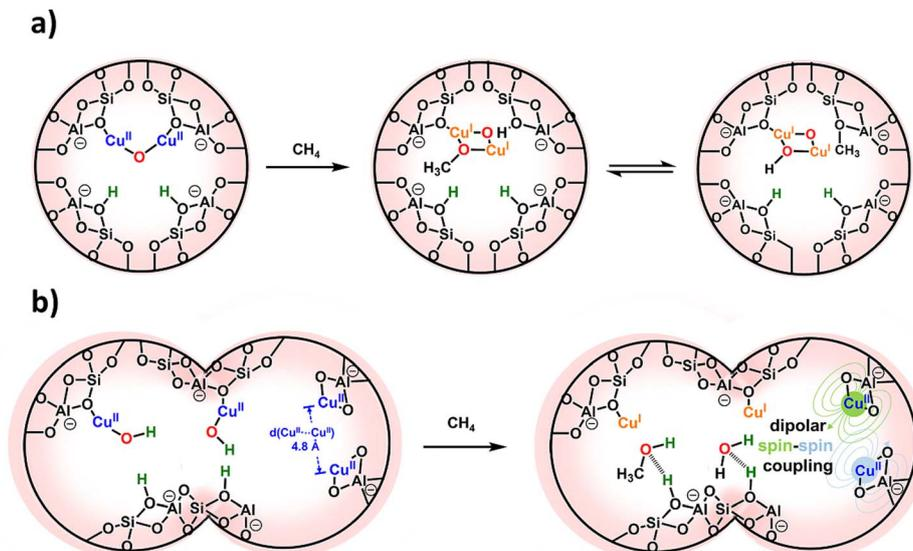
Fig. 14 Suggested reaction pathways of Cu–O species in Cu-MOR and their transformations during the reaction with CH<sub>4</sub>. (a) Pathway involving [Cu<sub>2</sub>(μ-O)]<sup>2+</sup> species. (b) Pathway involving [CuOH]<sup>+</sup> species, highlighting the inactivity of monomeric Cu species exhibiting dipolar spin–spin coupling at a separation distance of 4.8 Å.
