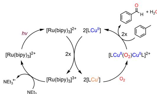
Scheme 12 Complex  $\text{LCu}(\text{I})$  ( $\text{L} = \text{tmpa}$  (tris(2-pyridylmethyl)amine)) after reaction with  $\text{O}_2$  according Göttlich and Schindler<sup>206</sup> and proposed general catalytic cycle for toluene oxidation (adapted from ref. 206).
