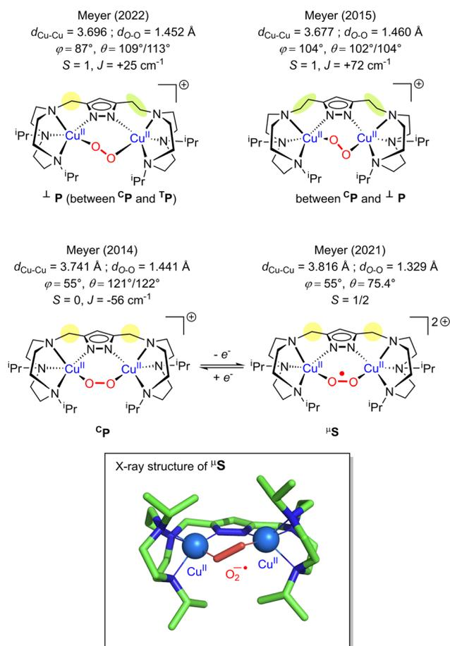
Fig. 8 Summary of the structurally characterized dicopper(II) peroxido species with pyrazolato/TACN based ligands from the Meyer group.<sup>160-162,167</sup>  $\varphi$  represents the torsion angle Cu-O-O-Cu and  $\theta$  the Cu-O-O angle.
