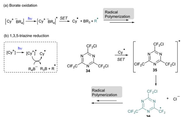
Scheme 9 Visible-light photopolymerization with cyanine: (a) borate oxidation; (b) 1,3,5 triazine reduction.
