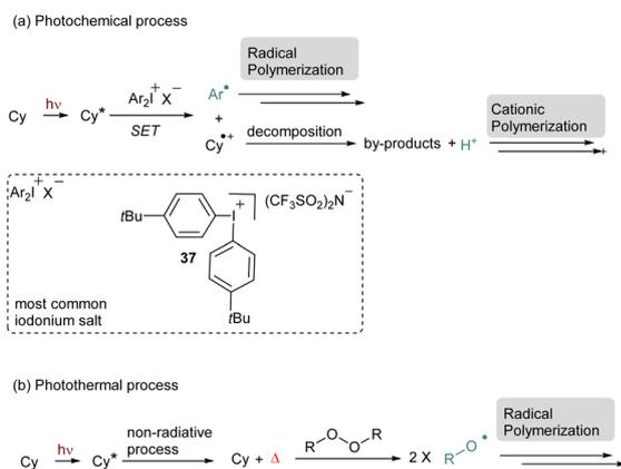
Scheme 10 General mechanism of NIR-polymerization with cyanines.
