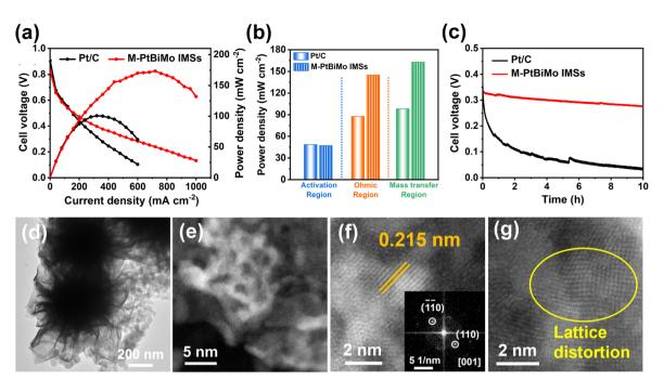
Fig. 5 (a) Polarization plots of M-PtBiMo IMSs and commercial Pt/C. (b) Qualitative analysis of power density, ohmic, and mass transfer of the overall performance. (c) Stability tests of M-PtBiMo IMSs and commercial Pt/C in MEA. (d-g) TEM and high-resolution HAADF-STEM images of M-PtBiMo IMSs after the durability test.
