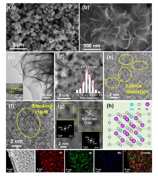
Fig. 1 (a and b) SEM images of M-PtBiMo IMSs. (c) TEM image of M-PtBiMo IMSs. (d) High-resolution HAADF-STEM image (the inset shows the column chart of the size of pores) of M-PtBiMo IMSs. (e and f) High-resolution TEM images of M-PtBiMo IMSs. (g) High-resolution HAADF-STEM image (the inset shows the corresponding FFT patterns) of M-PtBiMo IMSs. (h) Crystal structure. (i) HAADF-STEM pattern and element mappings of M-PtBiMo IMSs
