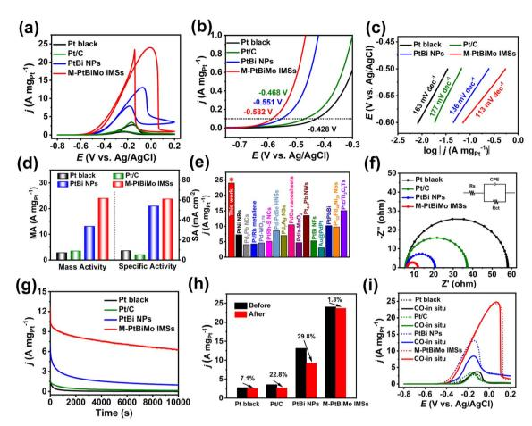
Fig. 3 (a and b) CV curves. (c) Tafel plots. (d) MA and SA. (e) Comparison of MA reported for various Pt/Pd-based EGOR catalysts. (f) Nyquist plots. (g) I-t curves recorded at -0.25 V. (h) Normalized MA of commercial Pt black, Pt/C, PtBi NPs, and M-PtBiMo IMSs before and after the I-t test. (i) CV curves of Pt black, Pt/C, PtBi NPs, and M-PtBiMo IMSs in CO-saturated electrolyte.
